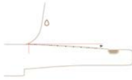
The cup dish has an inclination of 5° to let the coffee slip and go to the rail so that the coffee drops rest there
