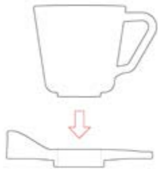
The cup fits in the dish, to hold and making it stable to move from one side to another
